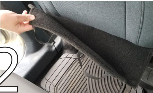
Unhook the flap behind seat that runs under bottom of the seat. You will need to unhook the plastic connector to release this flap.
