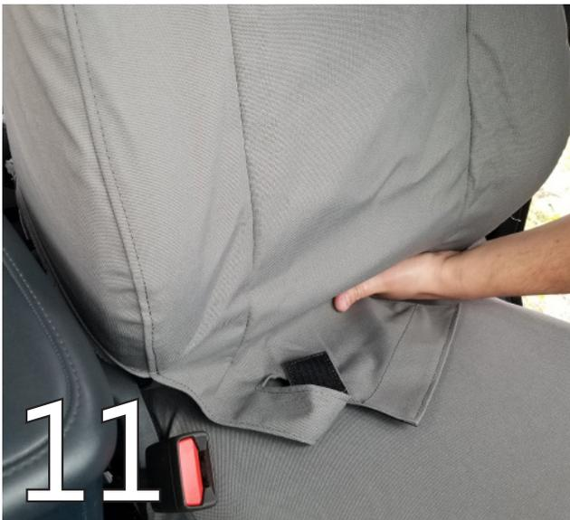
Push the flaps between the seat back and bottom as shown.
