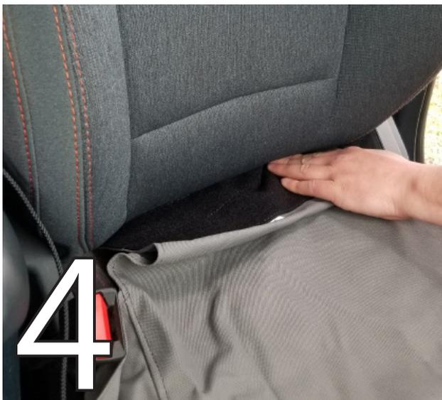
Push the flap between the seat back and seat bottom as shown.
