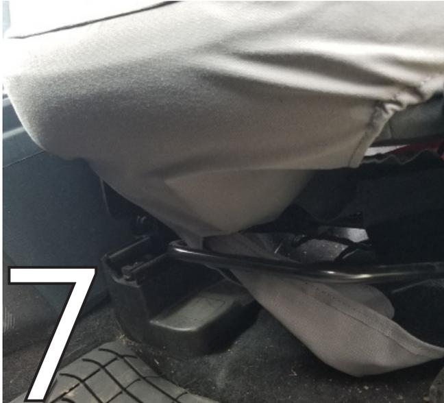
Run the flaps from the front to the back beneath the seat, making sure it runs above the adjustment bar and other seat mechanisms.
