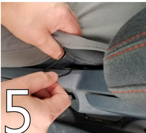
Drop the string closest to the door between the plastic trim and the seat cushion to run it on the inside of the seat frame. Drop the string on the other side down to the floor.
