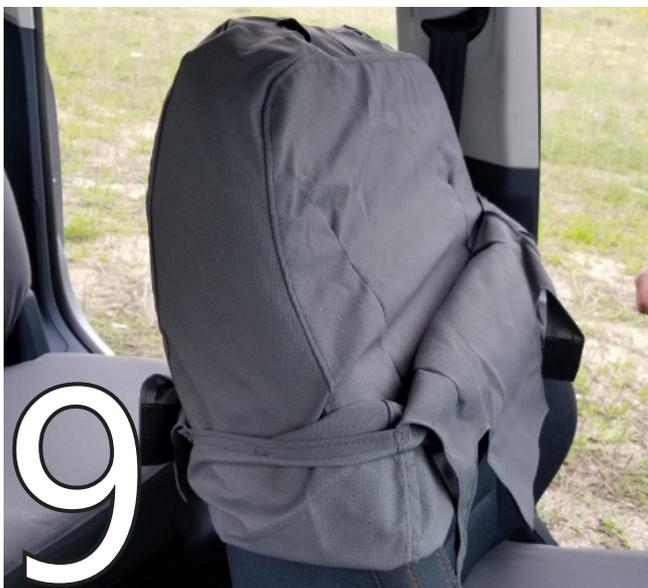
Turn the seat back partially inside out and slide it over the seat as shown.
